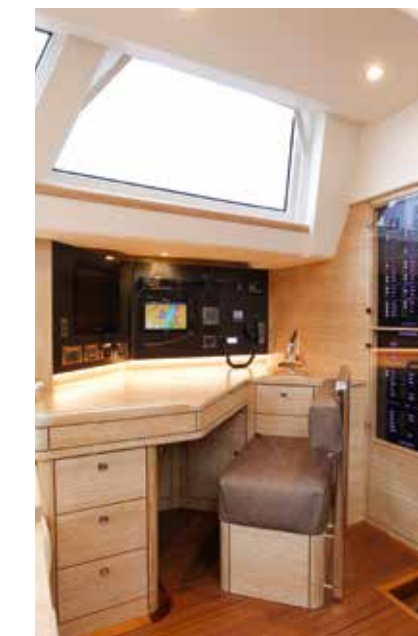
Above: The navstation is angled at 45 degrees with space for a rack of electronics
